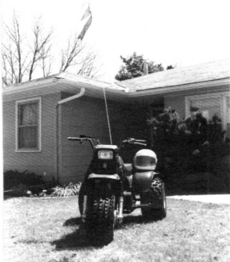
Figure 2. ATVs operating in state owned riding areas must have a 10' whip antenna with a bright red or orange flag.
